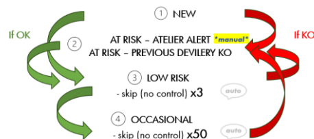
Figure 17. Scheme of the material control dynamic for material quality
